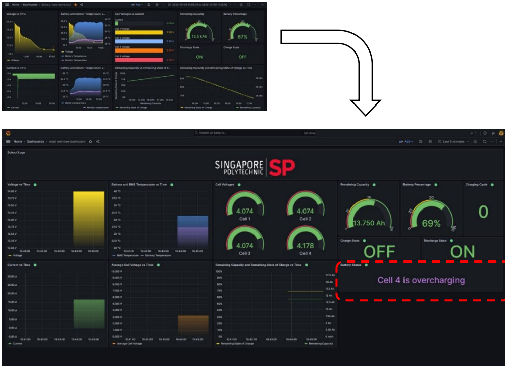
Figure 18: Addition of error detection algorithm
